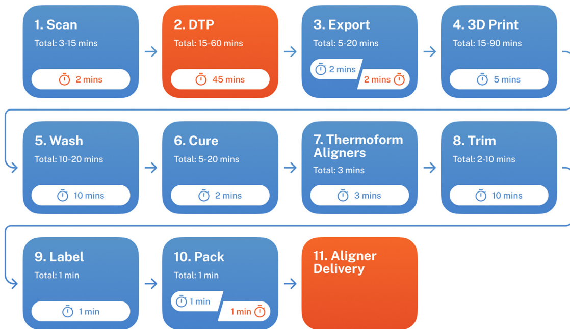
Fig. 1. A typical workflow for IHA fabrication with Orthodontist and Auxiliary roles and duration involved. Icons in orange indicate orthodontist role and in blue, auxiliary role. Watch icons indicate actual time spent by orthodontist/auxiliary as opposed to total time mentioned in individual boxes.
